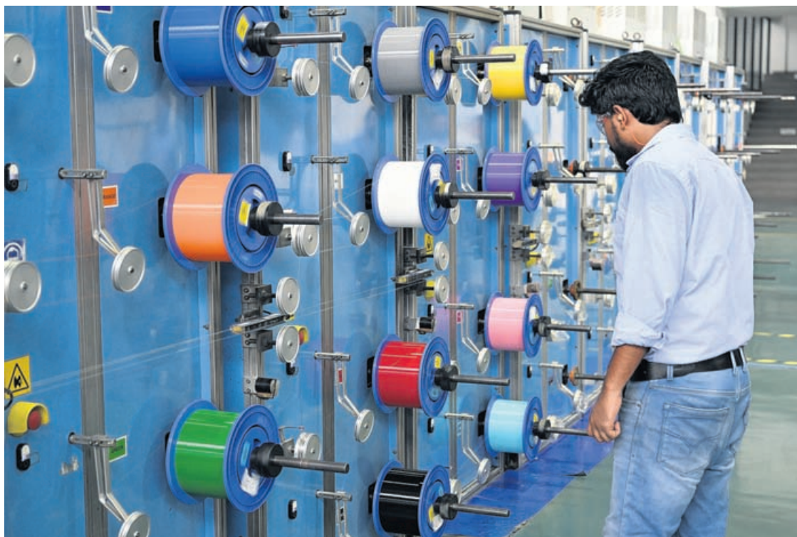
This photograph taken on July 9, 2026 shows a staff monitoring optical fibres being loaded onto spools at Sterlite Technologies Limited (STL) manufacturing facility in Maharashtra's Chhatrapati Sambhaji Nagar.
