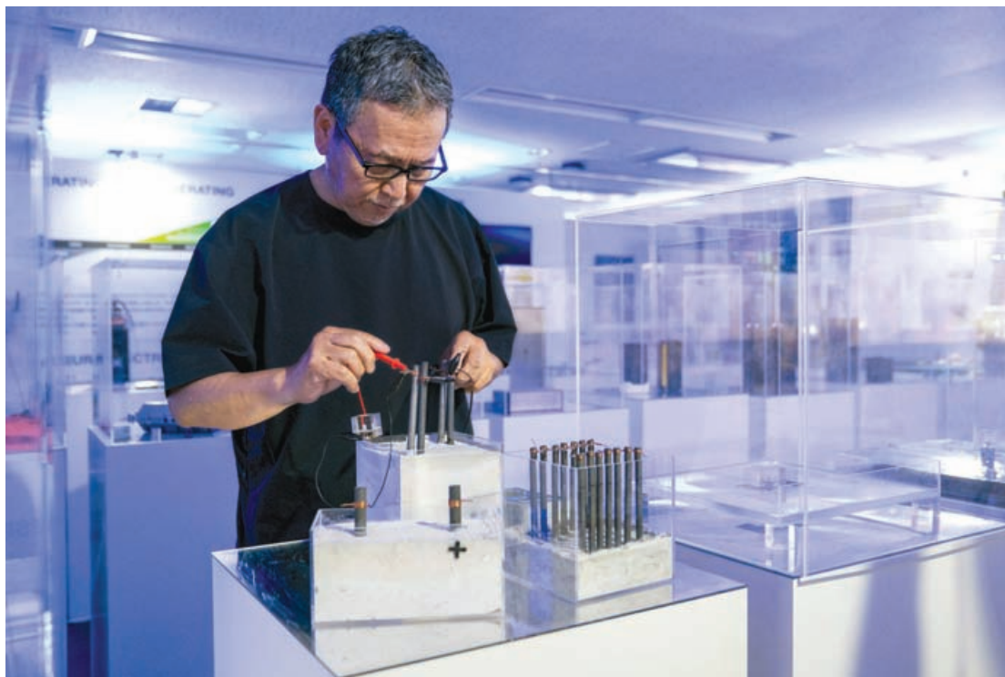
This photo taken on May 26, 2026 shows Japanese product designer and engineer Satoshi Nakagawa conducting an experiment to harvest electricity from a block of concrete at his laboratory in Tokyo.
