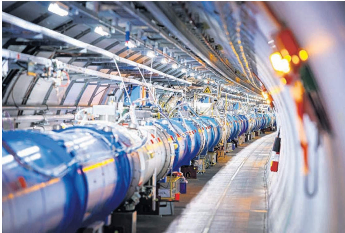
Some of the 1232 dipole magnets that bend the path of accelerated protons are pictured in the Large Hadron Collider (LHC) in a tunnel of the European Organization for Nuclear Research (CERN), during maintenance works on February 6, 2020 in Echevex, France, near Geneva.
