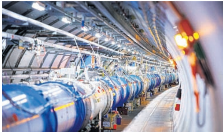
Some of the 1232 dipole magnets that bend the path of accelerated protons are pictured in the Large Hadron Collider (LHC) in a tunnel of the European Organisation for Nuclear Research (CERN), during maintenance works on February 6, 2020 in Echevex, France, near Geneva.
