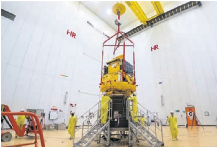
This photograph shows the Smile spacecraft (gold) fixed to a Vega-C rocket adaptor (black cone) on 25 March 2026, in Kourou, French Guiana, in preparation for liftoff from Europe's Spaceport.
