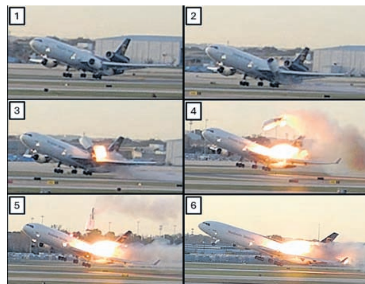
This combination photo provided by the National Transportation Safety Board (NTSB) via UPS shows a sequence of framegrabs made from video where an engine is seen detaching from the plane's left wing upon takeoff at the Louisville International Airport in Louisville, Nov. 4, 2025.
